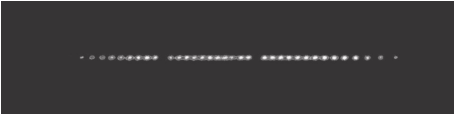
Figure 7.15. Image of fluorescence from about 40 trapped mercury ( ^{199}\text{Hg}^+ ) atomic ions. The ions are spaced by approximately 15 micrometers, and the two apparent gaps are different isotopes of mercury which do not respond to the probe laser. Reprinted courtesy of D. Wineland, at NIST.
