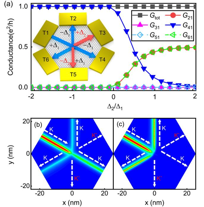
FIG. 5. (a) Dependence of current partitioning as a function of  $\Delta_2/\Delta_1$  for different output leads with Fermi energy  $E_F = 0.001t$ . Inset: Schematic of the six-terminal device with two pairs of gates labeled  $\Delta_1$  and  $\Delta_2$ . (b, c) Local density of states of incoming current at  $\Delta_2/\Delta_1 = 0.2$  and  $\Delta_2/\Delta_1 = 2$ , respectively, at the same Fermi level energies,  $0.001t$ .
